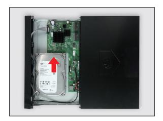
3 Holding the hard drive and the NVR, gently turn it over and line up the holes on the hard drive with the holes on the NVR. Using a screwdriver, screw the provided screws into the holes. Two groups of screw mounting holes are provided in the base frame of the NVR, respectively for installation of 3.5" hard drive and 2.5" hard drive. User should make selection based on their hard drive size. After complete HDD installation, assemble the cover.
