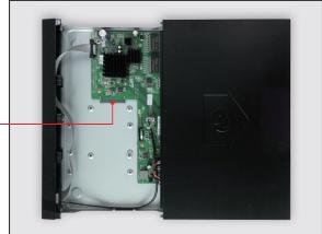
Connect data and power ports of hard drive to motherboard.
